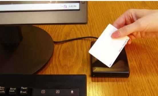
The Sphinx Logon Manager software turns an ID card or token into a secure two-factor computer authentication tool, and makes it easy to use strong passwords for logon processes.
